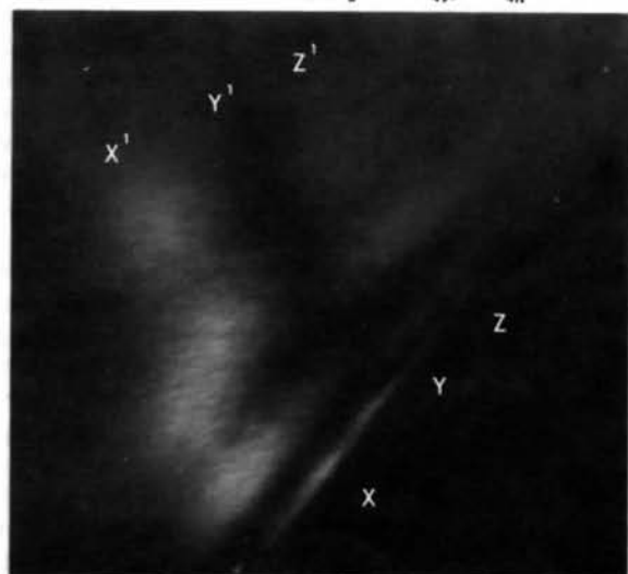
Fig. 10. Dark-field 210 image showing the edge of a \sigma particle with an orientation variation between b and \bar{b} of Fig. 8. The convergence used in taking this micrograph was approximately 0.5 mrad.
